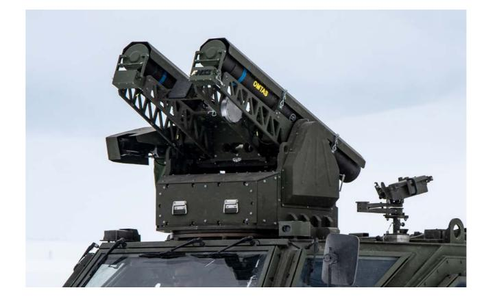
Capable of performing continuous 360 degrees traverse, the ARCT is armed with two anti-tank guided missiles along with a 7.62 mm coaxial machine gun. By means of its digital fire control system, the turret can automatically perform all the necessary ballistic calculations for achieving the highest hit probability, with both the missiles and coaxial machine gun. The gunner's sight system includes
